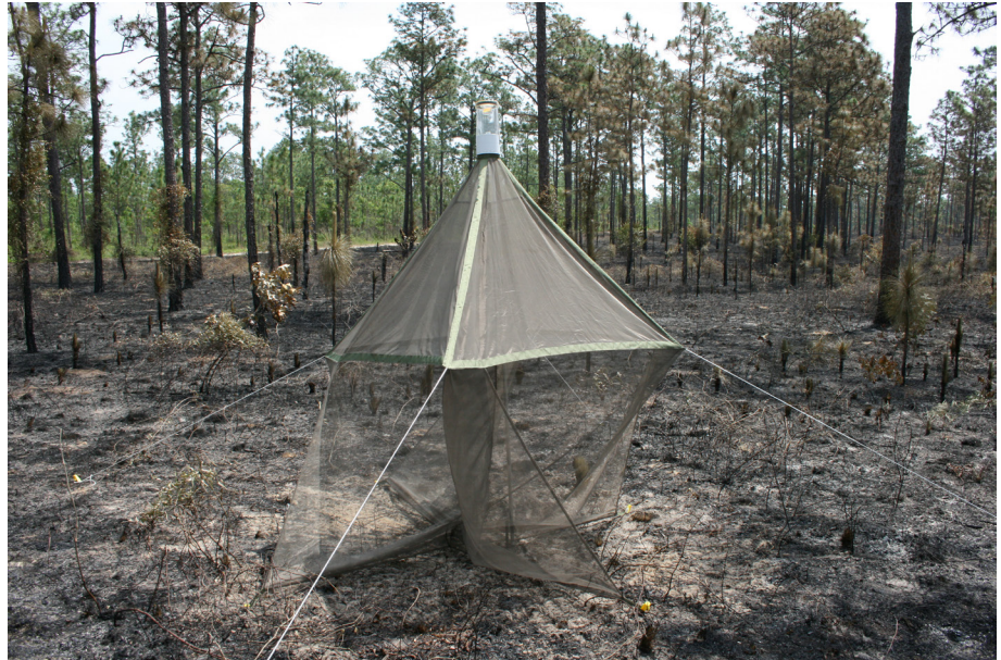
Figure 2. Malaise trap erected immediately after a prescribed fire in a longleaf pine forest. Traps were set up seven times in relation to each burn (before, during, immediately after, and then 2, 5, 10, and 12 months post-burn) to track the effects fire had on insect communities.
