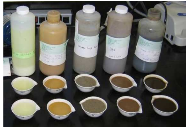
Figure 3. Various Co-substrates (left to right: whey, corn syrup, grease trap waste, dissolved air flotation, waste glycerine) Credit: Terrence Sauvé
