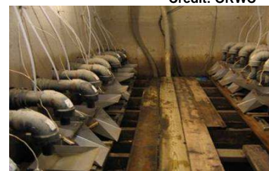
Figure 2. Land Application of Digestate on Experimental Plots at Campus d’Alfred and Collection System for Subsurface Drains
