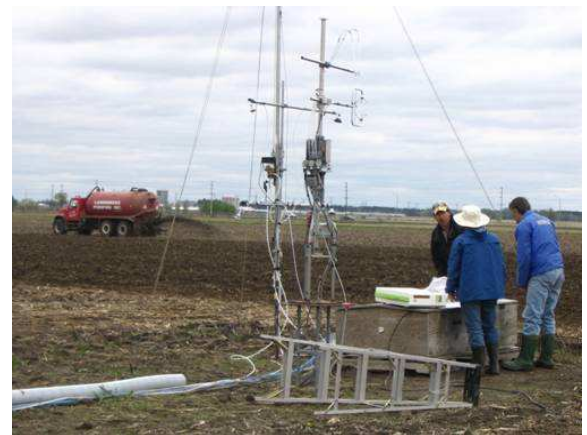
Figure 1. N 2 O & NH 3 Emission Measurements at Land Application of Raw Manure and Digestate (Dr. Pattey and AAFC staff)
