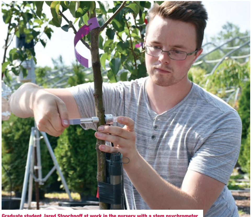
Graduate student Jared Stoochnoff at work in the nursery with a stem psychrometer.
