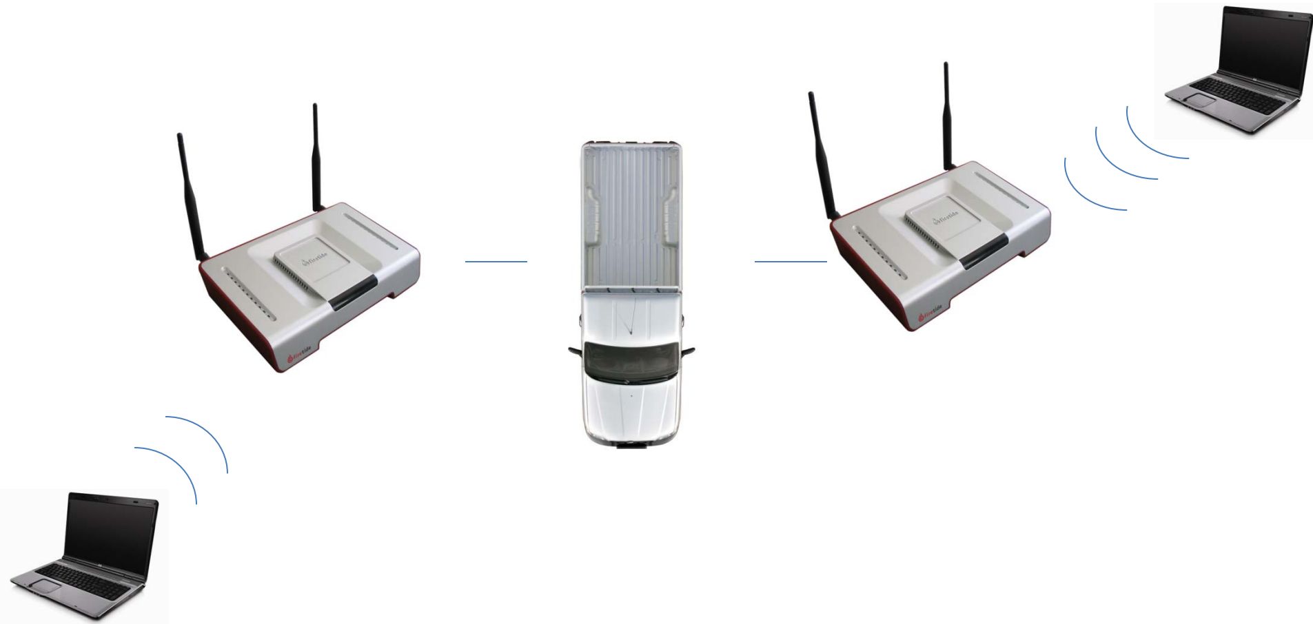
Obstruction between devices
