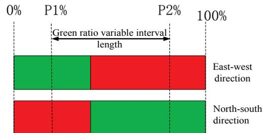
Figure 3. Intersections green ratio composition schematic.
