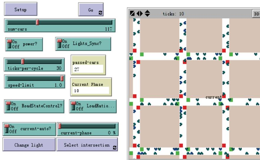
Figure 6. Traffic simulation system.
