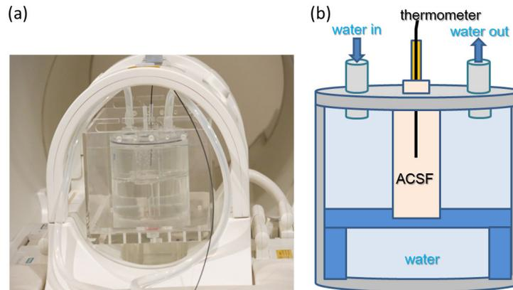
**Figure 1. Water-jacket-style thermal maintenance equipment. (a) Set in head coil of MRI scanner. (b) Graphical representation of the equipment.**
