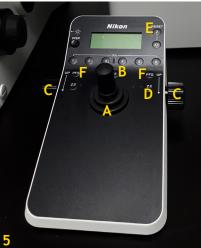
Using the focus wheels on the side of the Nikon controller box (Fig. 5C), move the objective nosepiece up until your sample is in focus (towards you = up, towards the wall = down). Switch to 'Fine Focus' by clicking on the 'Z' button on the controller box (Fig 5D). Fine and coarse focus are also indicated on the display ( $^{\land}$  ).
