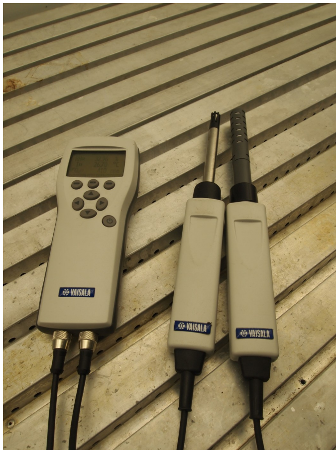
Vaisala M170 indicator (left) with HMP75 Temperature and Humidity Probe (middle) and GMP70 CO 2 Probe (right).
