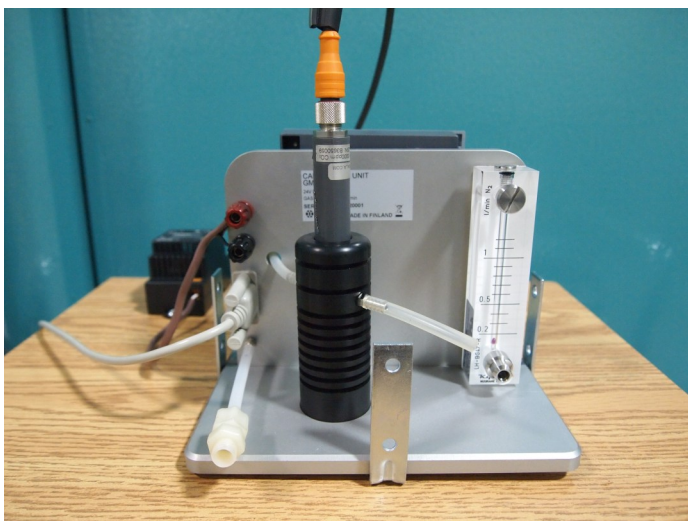
CO 2 sensor ready for recalibration using the Vaisala GMK220 calibration unit
