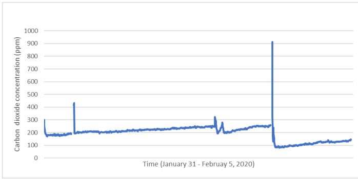
Figure 2: CO 2 concentration over time using the original scrubber design. Note the over compensation of the scrubber system after the large spike, likely caused by opening the chamber door for watering.
