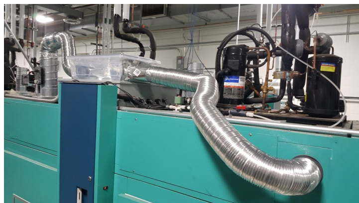
Figure 1a: Original CO 2 scrubber design with air moving horizontally through the box of soda lime and connected directly to the chamber inlet.
