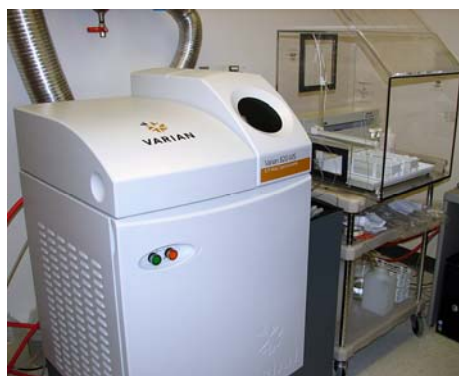
Figure 1. AHL ICP mass spectrometer, used for trace mineral panel and toxic metal panel for blood/serum, liver and feed samples.
