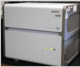
**Roche Lightcycler 480** instrument with computer and Lightcycler 480 block kit 96 – added another thermocycler to increase our capacity in this high-volume test area.
