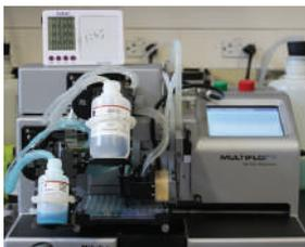
**BioTek Multiflow Fx microplate washer-dispensers and BioTek BioSpa 8 automated incubator** - links ELISA readers and imagers with washers and dispensers for full workflow automation for one of our highest volume tests, and as an economical replacement for our aging ELISA robot.
