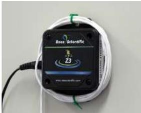
**Rees Scientific, Equipment Monitoring System (EMS)** – automated temperature monitoring system installed in 127 refrigerators, freezers, and incubators throughout building 89 in order to ensure reliable temperature control of equipment that is critical to laboratory operations.
