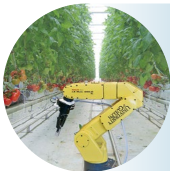
Robot harvester prototype for greenhouse use developed at U of G with Alliance funding
