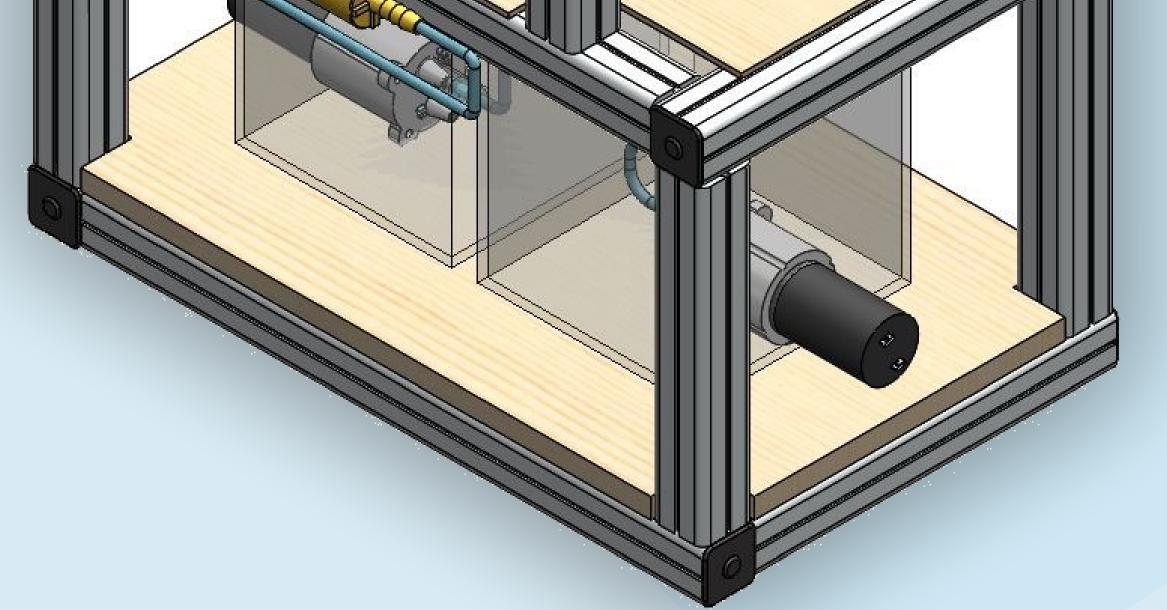
controlled by fluid flow rates. Temperature sensor input is fed to an Arduino microcontroller that uses pulse width modulation on two transistors acting as pump switches to determine flow rate.
