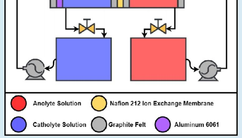
Detachable cut-off valves are used to stop fluid flow, allowing the system to be flushed with new chemicals when needed.
