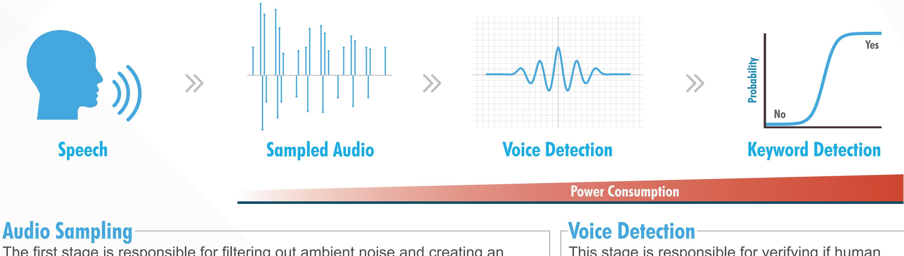
The first stage is responsible for filtering out ambient noise and creating an approximate digital signal from the analog audio. This is performed by creating an envelope around the amplified analog signal and only taking samples when
