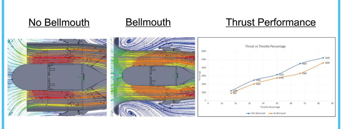
The addition of a bellmouth inlet improved thrust up to 36% and reduced noise.
