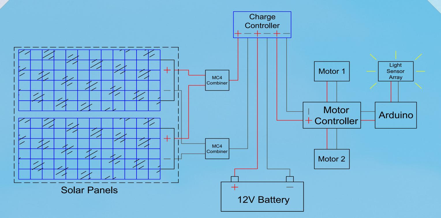
The design schematic highlights the two solar panels wired in parallel, connected to the charge controller which is subsequently routed to the control system array and back to the 12V battery.
