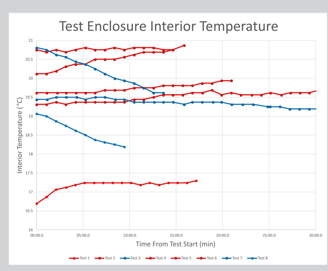
Climate control tests were conducted in a 64 ft<sup>3</sup> enclosure to determine the device effectiveness and the results showed that the average heating and cooling rates are 0.61 °C/hour and 0.51 °C/hour, respectively.
