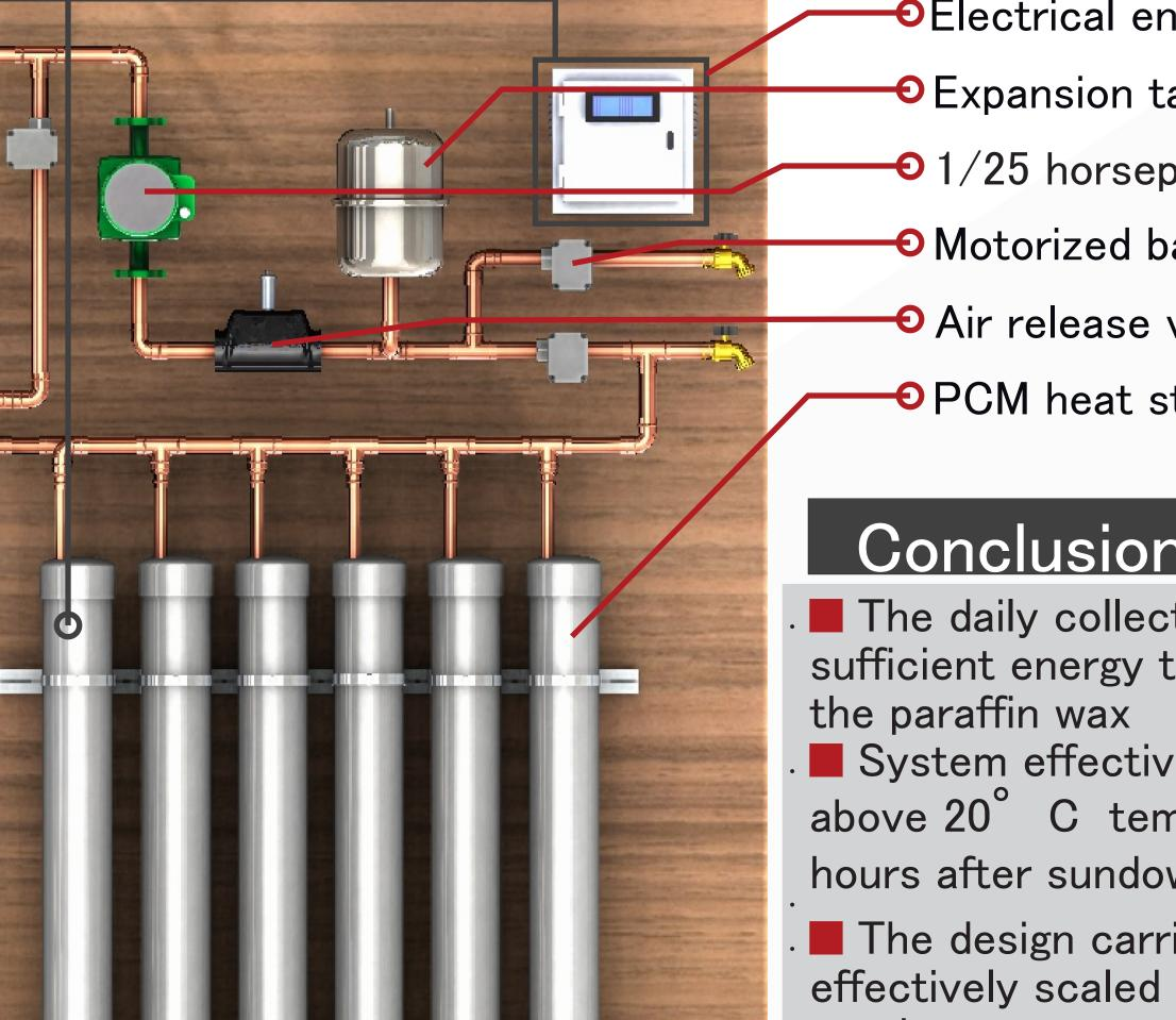
•Electrical enclosure box with lcd screen
