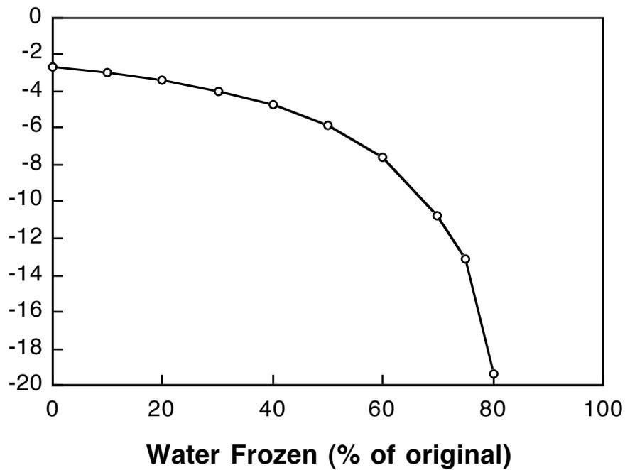
Freezing point depression curve for a mix with 10% NMS, 2% whey solids, 12% sucrose, 4% 42DE CSS, and 60% water (40% total solids).
