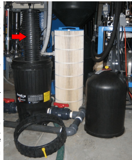
Fully disassembled: Red arrow indicates water distribution insert
