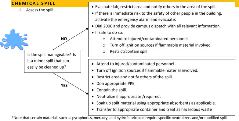
response procedures. Specific response procedures should be developed based on the identity and quantity of material being handled.
