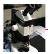
**Leica M80 Stereomicroscope** – in support of microscopy needs for microdissections and examinations, e.g., of honey bees.
