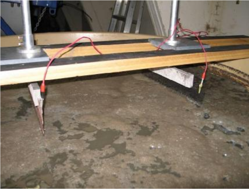
Figure 1. Electrodes mounted in configuration A; left: cathode (mild steel grid); right: anode (Ti/IrO 2 grid); direct electrical contact by alligator clips. Note that the electrodes are almost completely immersed in the liquid.
