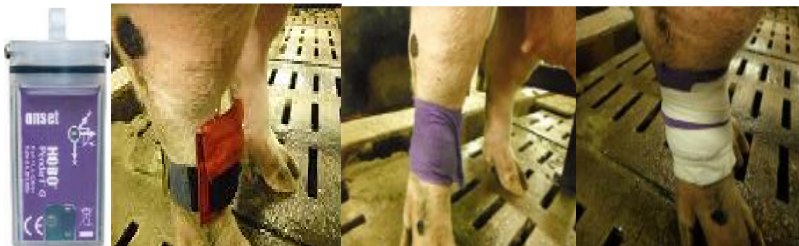
Figure 3. Fixing the accelerometer on the sow
