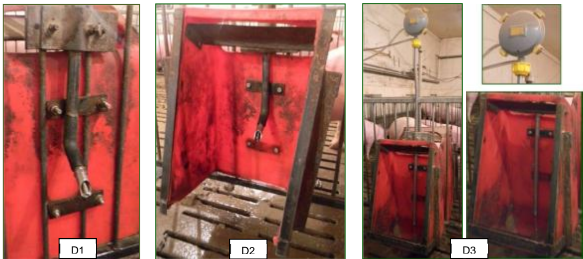
Figure 2. Three types of animal drinkers used: nipple (D1), nipple with side panel (D2) and a trough with side panel and constant water level (D3).
