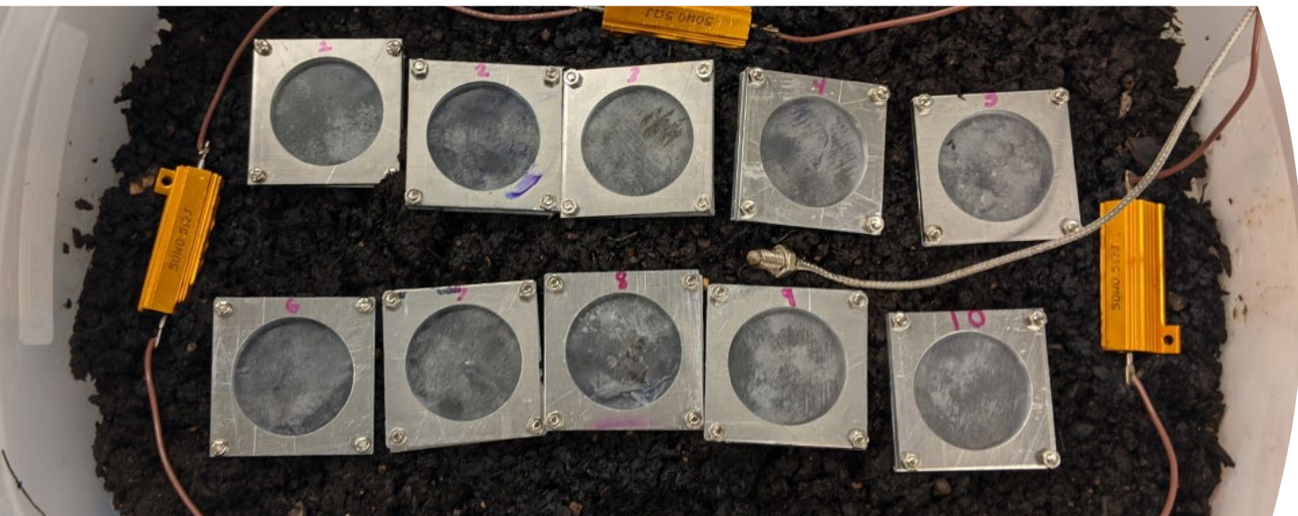
Biodegradability testing set-up in the Deiab Lab. Photo courtesy of Dr. Ibrahim Deiab
